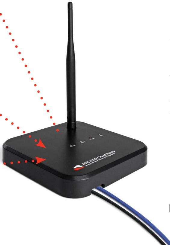
Taking cloud data logging to a whole new level! The **RFC1000 Cloud Relay** is a data logging hub that connects to the Internet via Ethernet and transmits data directly to the MadgeTech Cloud. This allows users to remotely monitor and manage groups of data loggers throughout a large facility or multiple locations without the need of a central PC.
