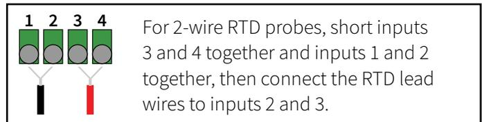
**Warning:** Note the polarity instructions. Do not attach wires to the wrong terminals. 100 Ω, 2 or 4 wire RTD probes are recommended for the most accurate performance. Most 100 Ω, 3 wire RTD probes will work, but MadgeTech cannot guarantee the accuracy. To determine whether or not the 3-wire RTD probe will work, the resistance between the two same colored wires should be less than 1 Ω. (Note: Please contact the manufacturer of the RTD probe for questions on the resistance.)
