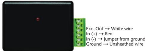
The diagram to the right outlines the wiring connections.
