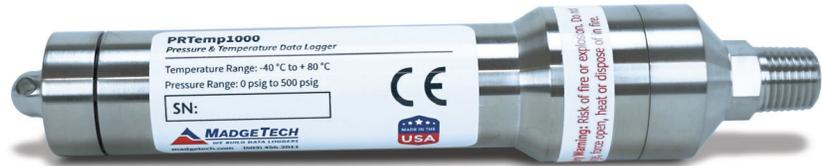
The PRTemp1000 is a rugged pressure recorder to accurately monitor and record pressure and temperature at user programmable reading intervals. The rugged stainless steel design allows for the device to be placed in harsh environments, which makes it well suited for use with air conditioning systems, chilled water, hot water, air, gas, oil and steam pressure systems.
