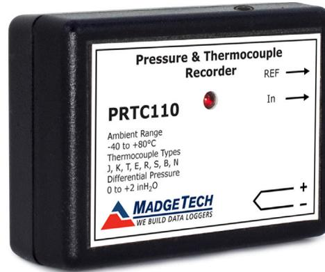
The PRTC110 is a differential pressure and temperature data logger, ideal for use in factory and laboratory applications. The device is available in a 0 to 2inH2O or 0 to 5inH2O model.
