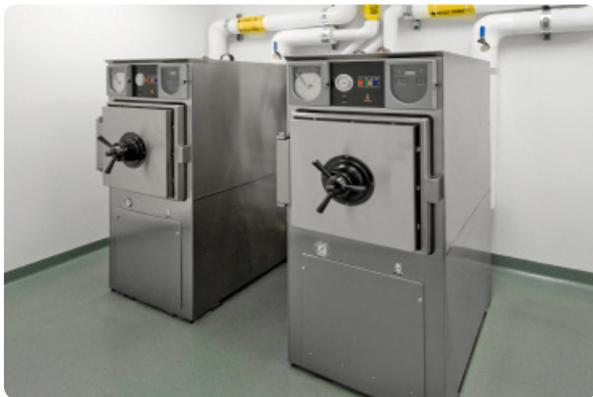
Freestanding autoclaves come in a variety of different door styles, ranging from single or double hinged doors to horizontal and vertical sliding and pocket doors.
