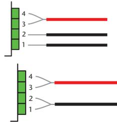
For 3-wire RTD probes, short inputs 3 and 4 together, then connect the lead wires to inputs 1, 2 and 3.
