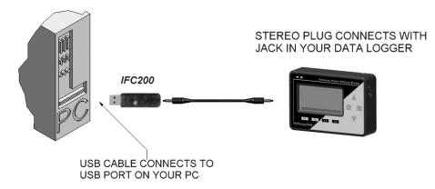
Fully insert the male connector of the IFC200 interface cable into the female receptacle of the data logger. Fully insert the female USB connector into the USB. (*Please see the Data Logger Software manual for further information.*)
