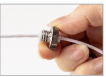
2. Thread the data logger probe through the thumb screw as shown.
