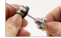
3. Insert data logger probe tip through the receptacle.
