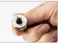
1. Ensure the sealing ferrule is seated inside the receptacle. Use the black rubber ferrule for 0.080 - 0.100 inch diameter probes or the red rubber ferrule for 0.100 - 0.125 inch diameter probes.
